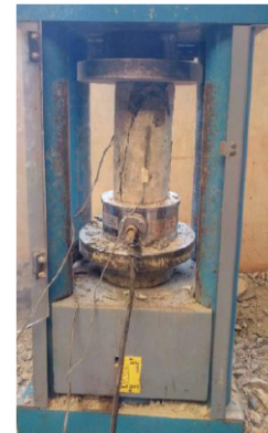
Fig. (5). Test of Static modulus of elasticity of CSMC.
