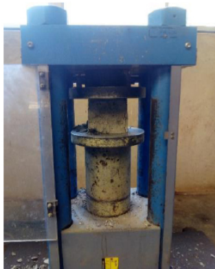
Fig. (3). Test of compressive strength of CSMC.
