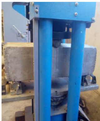
Fig. (4). Test of flexural strength of CSMC.
