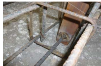
(b) Reinforcement detail of control specimen with bars welded to steel section.
