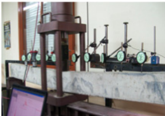
a). General view of the beam on the test bench
