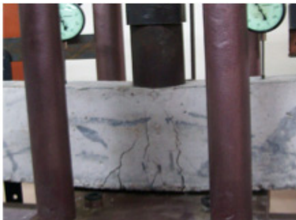
b). Crack pattern of the beam
