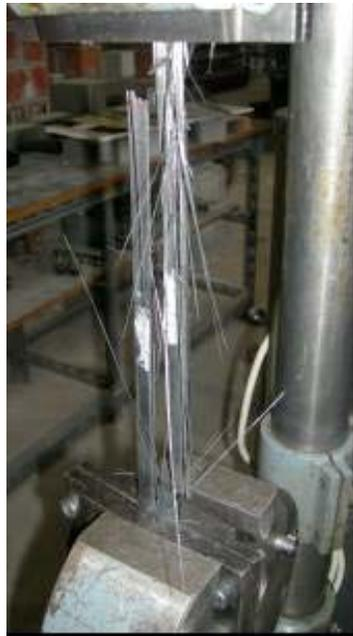
Fig. (3). CFRP specimen after tensile test.
