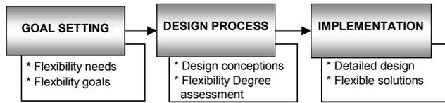
Fig. (2). A construction process that takes building flexibility into account consists of three distinct phases.
