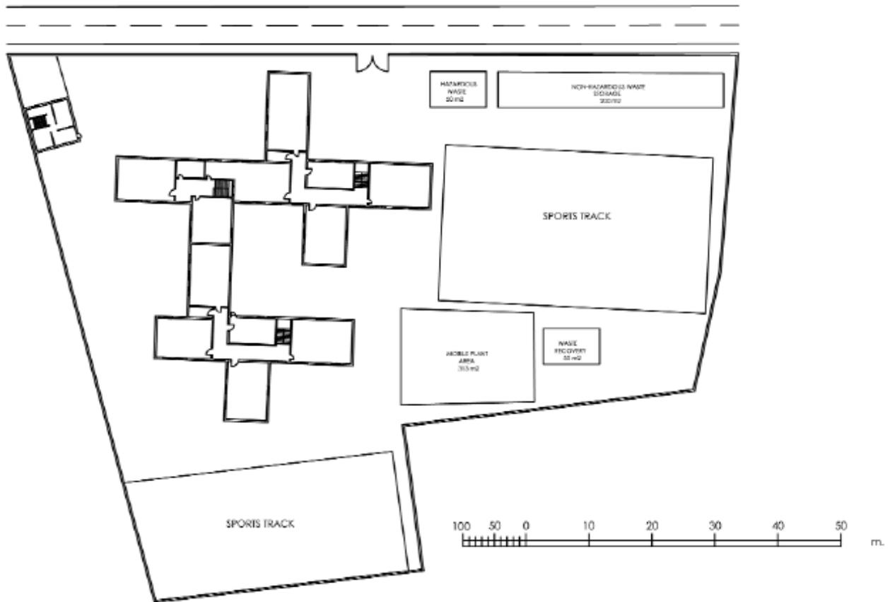
**Fig. (4).** The space needed for the C&D waste management: separation and in-situ treatment.
