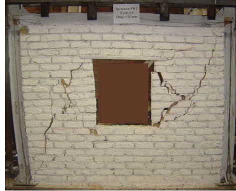
Fig. (7). Elements' failure points and crack patterns of the joints for specimen PW2 (numerical and experimental [19] results).
