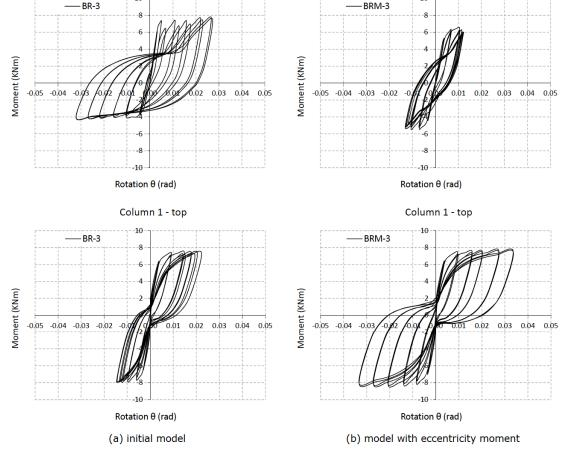
Fig. (9). Moment-rotation loops indicating reduction of plastic deformation at the beam and increase at the top column cross-section when eccentricity moment is applied.
