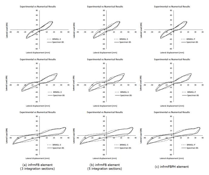
Fig. (11). Force-displacement loops of the frame (indicative loading cycles) for different numerical modeling approaches – comparison with experimental Specimen BS.
