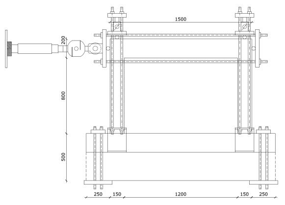
Fig. (2). Experimental setup to investigate the frame response under earthquake loading (dimensions in mm).
