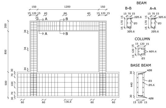
Fig. (1). Configuration and detailing of the examined 1/3 scale RC frames (dimensions in mm).
