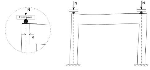
Fig. (7). Eccentric vertical loading of the columns.
