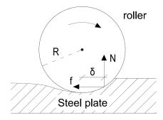
Fig. (5). Contact forces between a roller and a plate in pure rolling motion (after Lee *et al.* [25]).
