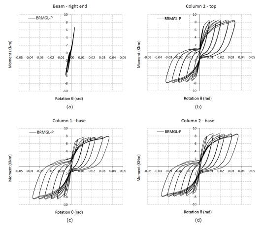
Fig. (13). Moment-rotation curves for beam and column cross-sections.
