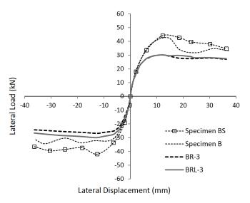
**Fig. (10).** Effect of beam axial loading on the response of the frame; model BRL-3 prevents beam tension during the analysis, resulting in increased frame strength.
