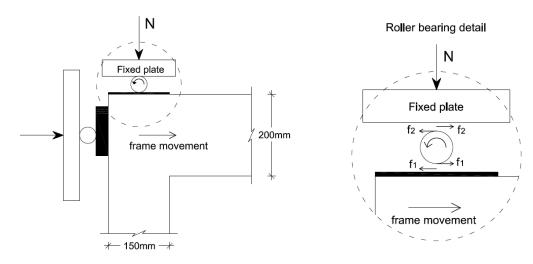
Fig. (6). Parasitic horizontal force f<sub>1</sub> on the beam-column joint due to roller friction forces.
