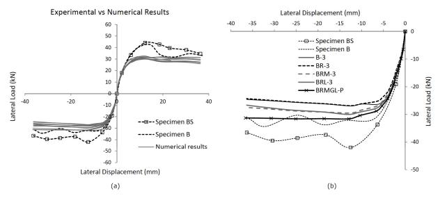
Fig. (12). Force-displacement curves; comparison between experimental and numerical results (a) several numerical approaches and (b) detail of selected analyses results.
