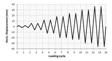
Fig. (3). Quasi-static cyclic earthquake loading program.
