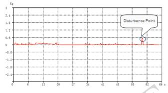
Fig. (7). Resistance at the speed of 0.1m/s in straight test mode.
