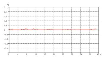
Fig. (10). Resistance at the speed of 0.1m/s in transverse test mode.
