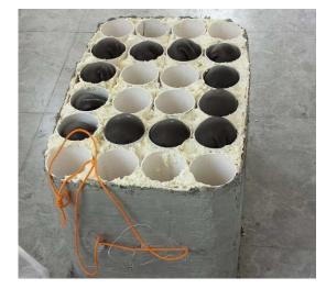
Fig. (4). The open caisson physical model.
