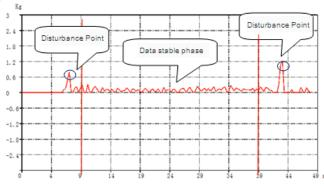
Fig. (9). Resistance at the speed of 0.3m/s in straight test mode.
