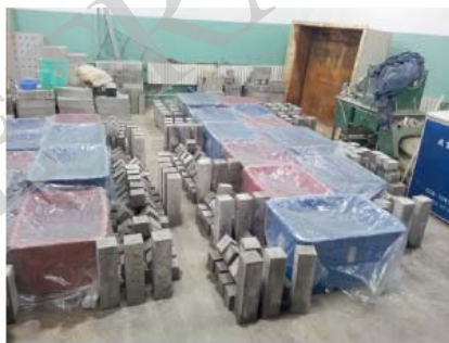
Fig. (1). Concrete specimens exposed to sulfate solution under drying-wetting cycles.
