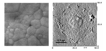
**Fig. (1).** SEM image of the surface of HAp sintered disk (Left panel), and AFM image of HAT-7 cell cultured on this surface (Right panel). The preparation of HAp sintered disks is described in Materials and Methods.
