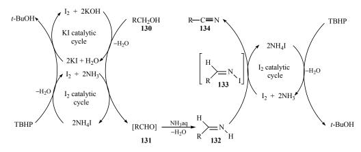
Scheme 24. Oxidative transformations of alcohols, aldehydes and amines using KI/I<sub>2</sub> -TBHP system.
