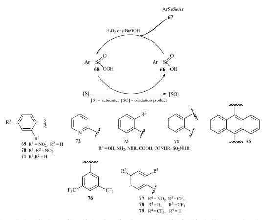
Scheme 17. The mechanism of hydroperoxide oxidation of organic substrate catalyzed by diaryl deselenide or areneselenenic acid.
