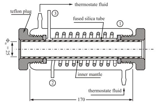
Fig. (1). Schematic representation of photochemical reactor (the dimensions are expressed in mm).
