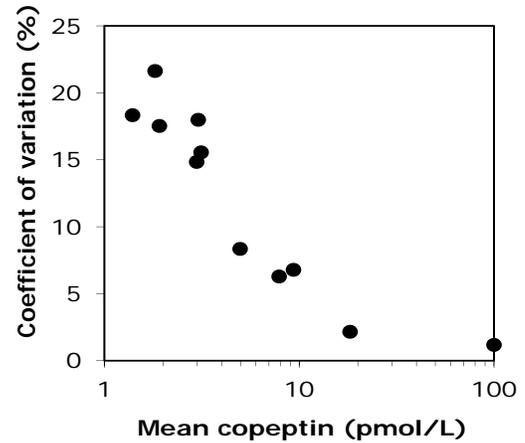
**Fig. (1).** Intra-assay imprecision of the copeptin US KRYPTOR assay. Patient serum or EDTA plasma samples with mean copeptin concentrations between 1.3-102 pmol/L were analyzed 10-22 times to determine the concentration-dependent intra-assay CV.
