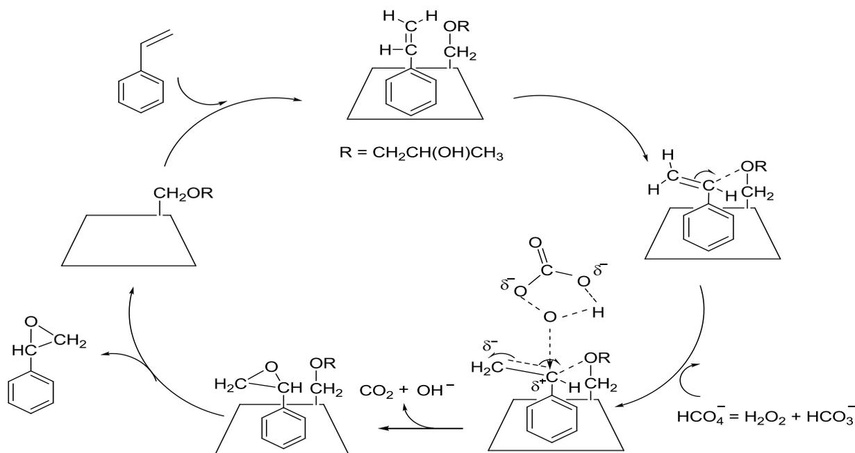
**Fig. (2).** Possible mechanism of the epoxidation of styrene in aqueous solution with the existence of 2-hp- $\beta$ -cyclodextrin.
