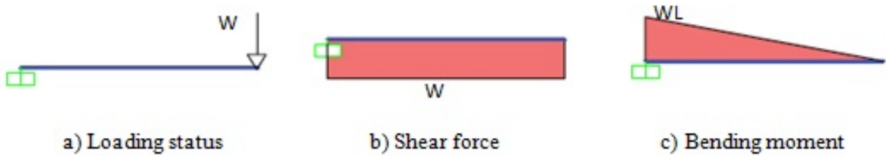
Fig. (4). Loading status, shear force and bending moment for cantilever beam.
