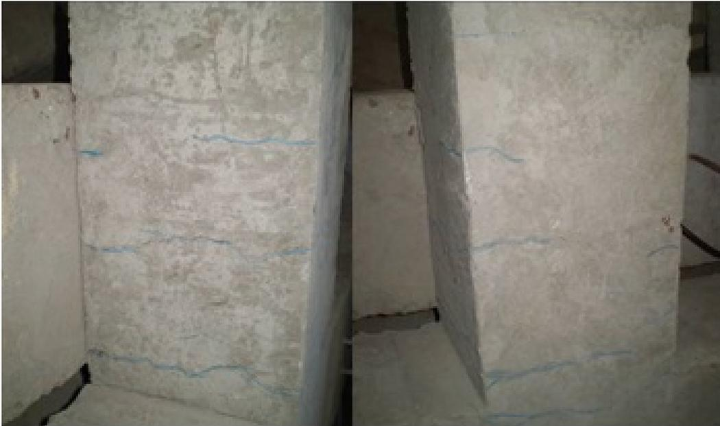
Fig. (9). Crack development of No.2 specimen in the cyclic load.
