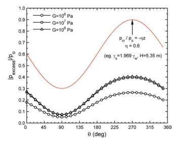
Fig. (15). The distribution of  $|p_{\text{excess}}|/p_o$  around pipe perimeter for various *G*. ( $K_0$ =0.5,  $\gamma_s$ =1.969 $\gamma_w$ , *H*=5.0 m).
