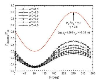
Fig. (24). The distribution of  $|p_{\text{excess}}|/p_{\text{o}}$  around pipe perimeter for various w/D.
