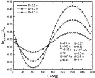
Fig. (26). The distribution of  $|p_{\text{excess}}|/p_0$  around pipeline circumference for various pipe diameters.
