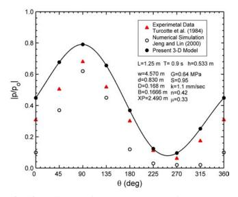
Fig. (6). Verification of numerical simulations from the present model against experimental data in Turcotte *et al.* [23] for short wave lengths.
