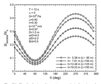
**Fig. (31).** The distribution of  $|p_{\text{excess}}|/p_0$  around pipeline circumference for various water depths.
