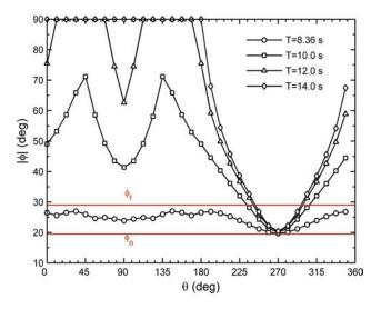
Fig. (30). The distribution of  $|\phi|$  around pipeline circumference for various wave periods.
