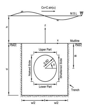
**Fig. (1).** Definition sketch: cross-section of a trenched submarine buried pipeline.
