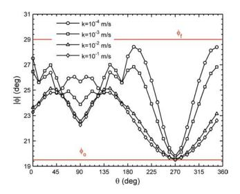
**Fig. (18).** The distribution of  $|\phi|$  around pipeline perimeter for various *k* ( $K_0$ =0.5,  $\gamma_s$ =1.969 $\gamma_w$  and *H*=5.0 m).
