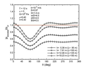
Fig. (32). The potential of soil liquefaction around pipe perimeter for various h ( $K_0 = 0.5$  and  $\gamma_s = 1.969\gamma_w$ ).
