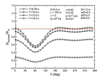
Fig. (29). The potential of soil liquefaction around pipe perimeter for various *T*. ( $K_0 = 0.5$  and  $\gamma_s = 1.969\gamma_w$ ).
