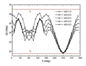
**Fig. (23).** The distribution of  $|\phi|$  around pipeline circumference for various *d/D*.
