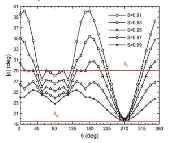
**Fig. (20).** Variations of  $|\phi|$  with soil saturation.
