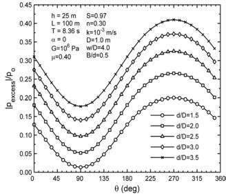
**Fig. (21)**. The distribution of  $|p_{\text{excess}}|/p_{\text{o}}$  around pipeline circumference for various d/D.
