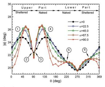
Fig. (13). The distribution of stress angle amplitude  $(|\phi|)$  around pipe circumference for various wave directions (soil, wave and pipe properties are as in Fig. (12)).
