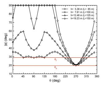
**Fig. (33).** The distribution of  $|\phi|$  around pipeline for various water depths.
