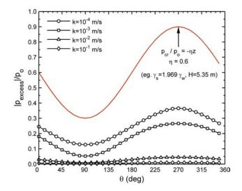
**Fig. (17)** The distribution of  $|p_{\text{excess}}|/p_0$  around pipe perimeter for various *k*.
