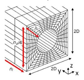
**Fig. (4).** Definition Sketch: 3-D Finite Element Mesh in the vicinity of pipeline.
