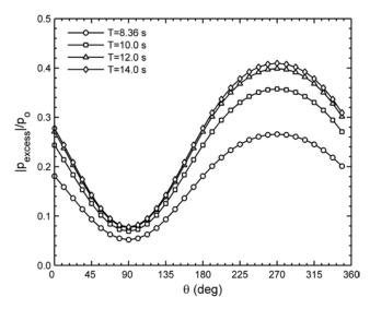
**Fig. (28).** The distribution of  $|p_{\text{excess}}|/p_0$  around pipe perimeter for various *T*.
