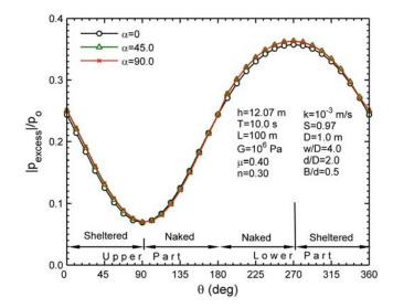
Fig. (14). The distribution of amplitude of wave-induced excess pore pressure  $(|p_{\text{excess}}|/p_o)$  around pipe circumference for various wave directions.
