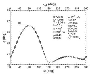
**Fig. (12).** The distribution of stress angle for a point located on the pipe perimeter at  $\theta$ =135° (a) over a pipeline span axis, when *t*=*T* (see the upper horizontal axis:  $\kappa_y y$ ), (b) over a wave period, when *y*=0 (see the lower horizontal axis:  $\omega t$ ).
