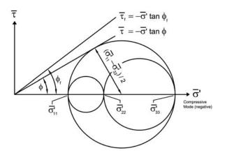
Fig. (9). The Mohr-Coulomb shear failure criterion.
