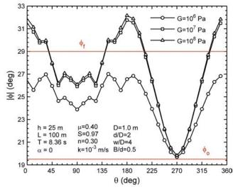
Fig. (16). The distribution of  $|\phi|$  around pipe circumference for various *G* ( $K_0$ =0.5,  $\gamma_s$ =1.969 $\gamma_w$ , *H*=5.0 m).
