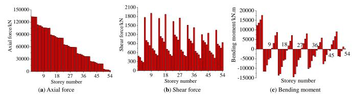
Fig. (14). Internal forces of right-side mega column under P+V+H.
