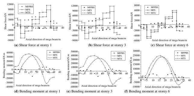
Fig. (30). Comparison of internal forces in mega beam among three systems.
