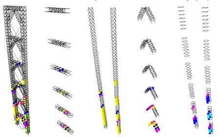
(a) whole (b) giant beams (c) braces between mega column limbs (d) mega Λ-shape steel bracing truss (e) floor beams between mega column limbs
