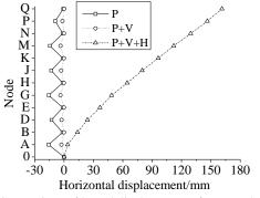
Fig. (12). Comparison of lateral displacement of mega column.
