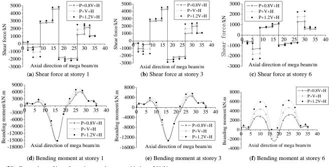
Fig. (20). Comparison of inter forces in mega beam considering  $\pm 20\% V$ .
