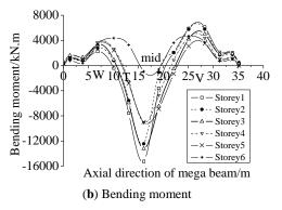
Fig. (15). Internal forces in mega beam under P+V+H.
