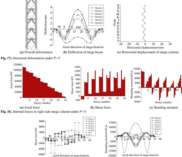
(a) Shear force (b) Bending moment Fig. (9). Internal forces in mega beams under P+V.
