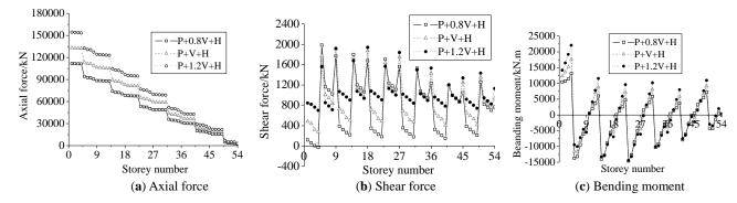
Fig. (19). Comparison of internal forces in right-side mega column considering  $\pm 20\%$ V.
