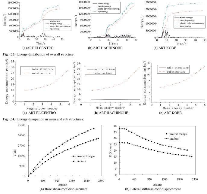
Fig. (35). Base shear and lateral stiffness
