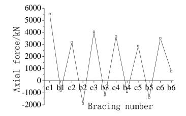
Fig. (6). Internal force of composite bracings at the prestress state.
