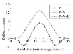
Fig. (13). Comparison of vertical displacement of mega beam.
