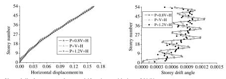
Fig. (17). Comparison of lateral displacement and storey drift ratio considering  $\pm 20\%$ V.
