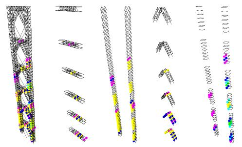
(a) whole (b) mega beams (c) braces between mega column limbs (d) mega A-shape steel bracing truss (e) floor beams between mega column limbs
