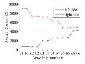
Fig. (16). Internal forces of composite bracings under P+V+H
