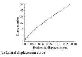
Fig. (11). Lateral displacement and storey drift ratio under P+V+H.
