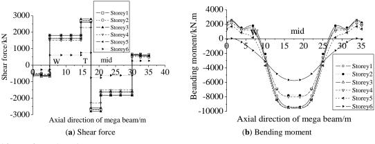
Fig. (5). Internal forces of mega beam in prestress state.
