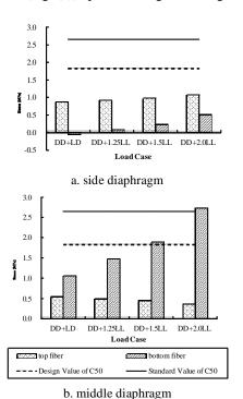
Fig. (3). Concrete stress of mid-span diaphragm under different live
