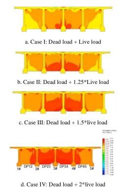
Fig. (2). Stress of concrete under different live load intensity.
