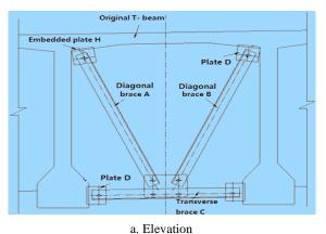
Fig. (4). Design of spacial Double-K shape brace.
