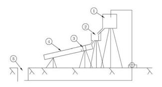
Notes: (1) Mud storage tank; (2) Pressure stabilizing tank; (3)Energy dissipation fence; (4)Straight flume; (5)Mud mixing pool.
