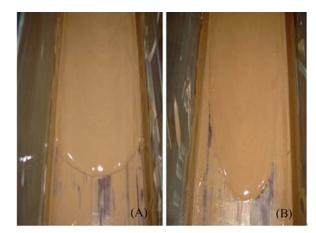
Notes: (A) Fixed bed and gentle slope (i = 5.5%,  $\gamma = 16.8$  KN/m3); (B) Fixed bed and steep slope (i = 5.5%,  $\gamma = 16.8$  KN/m3).
