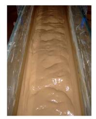
Notes: Fracture state of mud surface ( $\gamma = 17.5$  KN/m3, i = 14.0%, Q=1.50 l/s).
