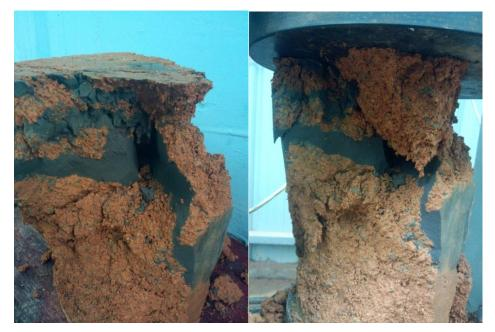
Fig. (11). Slurry veins inside the medium.
