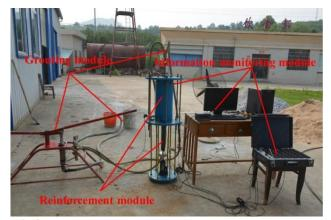
Fig. (9). Structure of model experiment device
