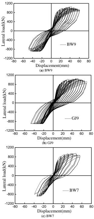
Fig. (5). Load-displacement hysteretic loops of specimens.
