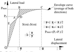
Fig. (7). Displacement ductility parameters.
