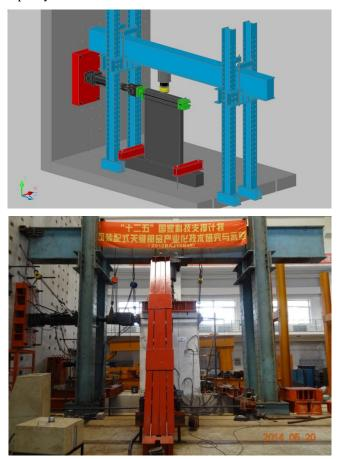
Fig. (3). Schematic representation of loading frame.
