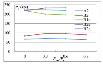
Fig. (6). Effect of preload level on ultimate load-carrying capacity.
