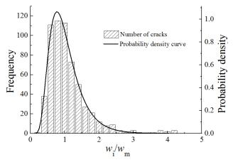
Fig. (11). Crack width frequency distribution.
