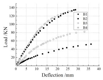
Fig. (7). Mid-span load-deflection curves.
