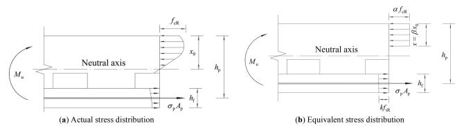
Fig. (12). Stress distribution on a cross section of the specimen at the ultimate moment.
