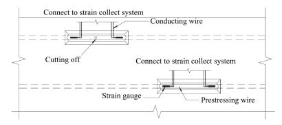
Fig. (5). Measurement of the effective prestress.
