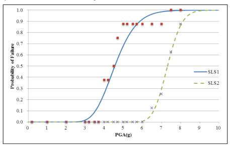
Fig. (12). Seismic fragility curve of the anchor bolt considering shear failure.
