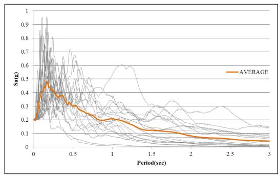
Fig. (6). Acceleration response spectrum.
