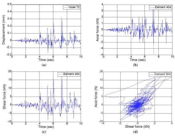
Fig. (10). Response time histories: (a) displacement at the top of the BOG compressor, (b) axial force in an anchor bolt, (c) shear force in an anchor bolt, and (d) shear force-tension diagram.
