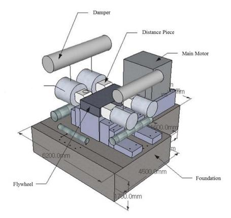
Fig. (3). Mimetic diagram of the BOG compressor.
