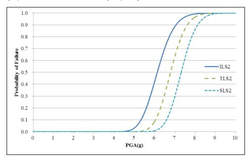
Fig. (15). Seismic fragility curves of the anchor bolt considering ultimate failure criteria.
