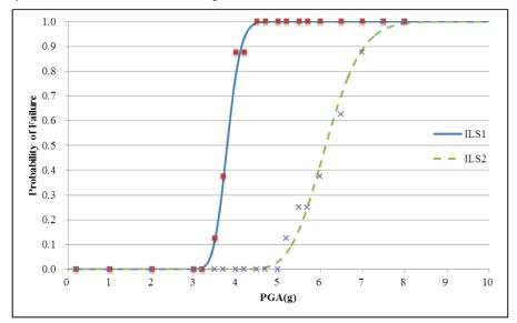
Fig. (13). Seismic fragility curve of the anchor bolt considering the shear-tension interaction failure.
