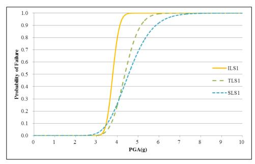
Fig. (14). Seismic fragility curves of the anchor bolt considering the yielding failure criteria.
