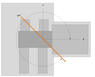
Fig. (7). Direction of the seismic load application to the BOG compressor.
