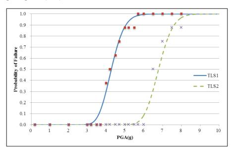
Fig. (11). Seismic fragility curve of the anchor bolt considering tension failure.
