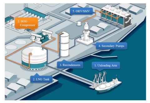
Fig. (1). Concept map of an LNG receiving terminal.
