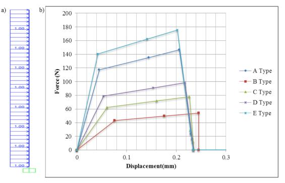
Fig. (5). Pushover result of anchor bolt : a) distributed load (N) and b) pushover result.
