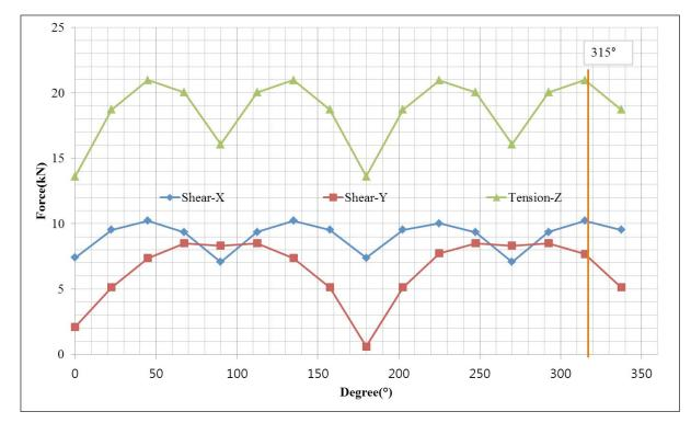
Fig. (8). Forces in the anchor bolts due to variations in the seismic loading direction.
