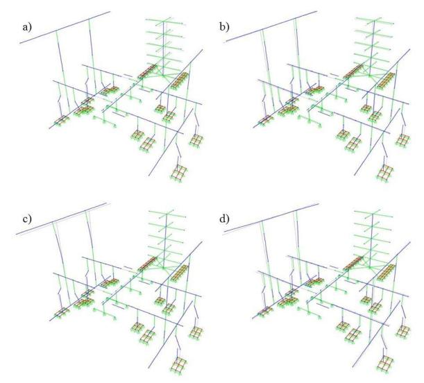
Fig. (9). Modal analysis of BOG compressor : a) mode 1 (0.048 sec), b) mode 2 (0.038 sec), c) mode 3 (0.035 sec), and d) mode 4 (0.032 sec).
