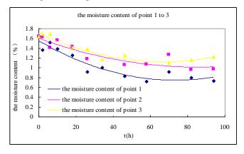
Fig. (7). The changes of moisture content with time at the surface of sludge.
