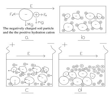
Fig. (9). The process of electro-osmosis dewatering.
