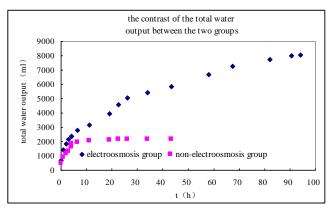
Fig. (12). The contrast of the total water output between the two groups.
