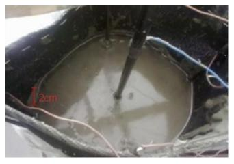
Fig. (10). the phenomenon of water concentrating on the surface of sludge.
