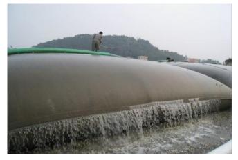
Fig. (2). Sludge dewatering by the geotube.
