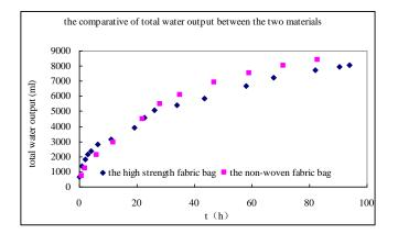
Fig. (13). The contrast of the total output water between the two materials.
