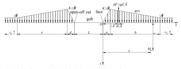
Fig. (2). Analysis of mining floor stress distribution during the first weighting of main roof.
