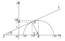
Fig. (3). The Mohr-Coulomb criterion in coordinates  $\sigma - \tau$
