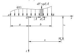
Fig. (1). Schematic diagram of distributed load on semi-infinite plane.
