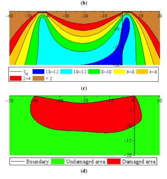
Fig. (4). The stress contour and mining damage area of floor strata.
