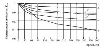
Fig. (2). Relationship between the *RubCon* coefficient of chemical resistance and time of corrosion medium exposition: 1- water, 2-30% solutions of sulfuric acid, 3-36% solutions of hydrochloric acid, 4-10% solutions of caustic soda, 5- diesel fuel, 6-5% solutions of acetic acids.
