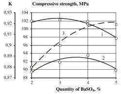
Fig. (5). Impact of  $BaSO_4$  quantity on *RubCon* compressive strength operated in no aggressive environments (line 1), compressive strength (line 2) and resistance coefficient (line 3) after 90 day's exposition into 36% solution of HCl.
