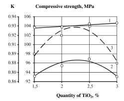
**Fig. (4).** Impact of  $TiO_2$  quantity on *RubCon* compressive strength operated in no aggressive environments (line 1), resistance coefficient (line 2) and compressive strength (line 3) after 90 days exposition into 36% solution of HCl.
