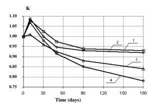
Fig. (7). The coefficient chemical resistance dependence of the exposure time; 1 - 70 %- solution of H<sub>2</sub>SO<sub>4</sub>; 2 - 5 %- solution of H<sub>3</sub>PO<sub>4</sub>; 3 - 25 %- solution of NH<sub>4</sub>OH; 4 - 36 %-solution of HCl.
