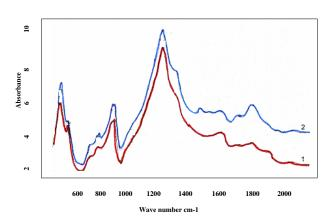
**Fig. (9).** Specters of *RubCon*: 1- before  $\gamma$ -exposition, 2- after  $\gamma$ -exposition.
