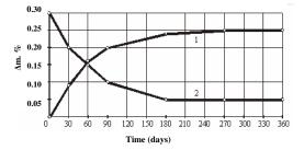
**Fig. (6).** 1- Water absorbing of fiber reinforced *RubCon*; 2-Coefficient of water resistance depending on exposure duration into water.
