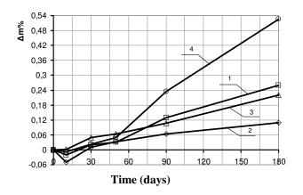
**Fig. (8).** Kinetics of mass-absorption of *RubCon* : **1** - 70 %-th solution of a sulfuric acid; **2** - 5 %-th solution of a phosphoric acid; **3** - 25 %-th water solution of ammonia; **4** - 36 %-th solution of a hydrochloric acid.
