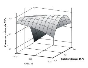
**Fig. (3).** Compressive strength of *RubCon* samples relationship between quantities of altax and sulfur + tiuram-D after exposition in 36% solution of a hydrochloric acid.
