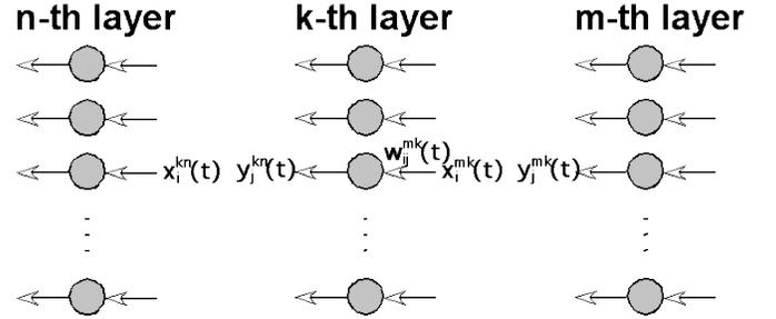
**Fig. (3).** Schematic diagram showing the network connectivity at the  $k$ -th layer, connecting from the  $m$ -th layer to the  $n$ -th layer.
