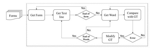
Fig. (4). General verification flowchart for the Online-KHATT database.
