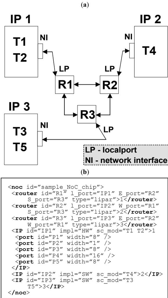
Fig. (3). Sample target NoC architecture scheme (a) and corresponding system\_noc.xml (b).
