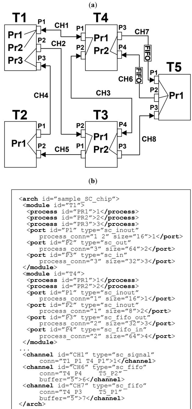
Fig. (2). Sample SystemC architecture scheme (a) and part of corresponding *system\_sc.xml* (b).
