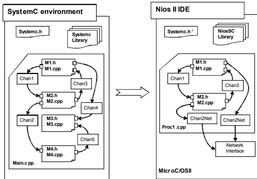
Fig. (4). Embedded software generation.
