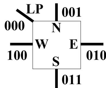
Fig. (13). Designation of router ports.
