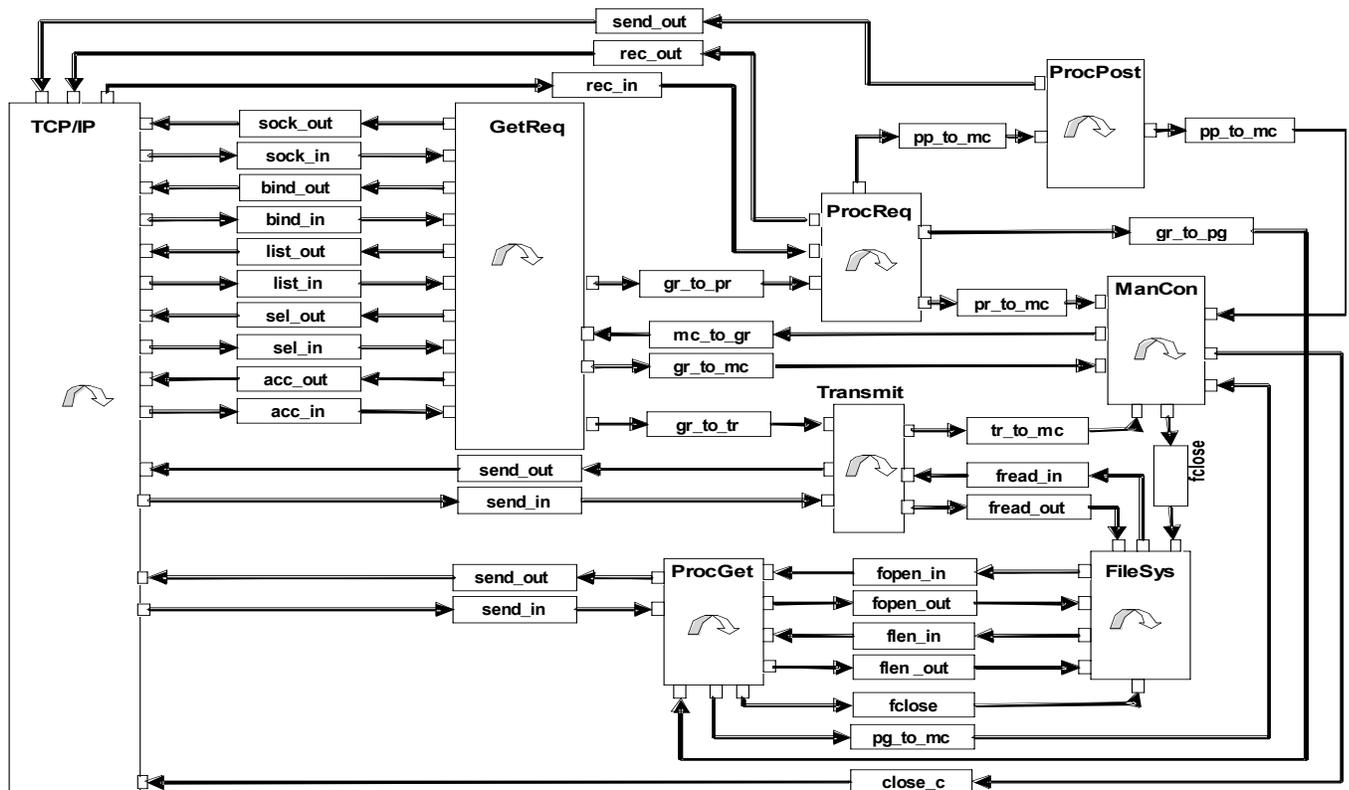
Fig. (10). SystemC architecture scheme of the WWW server.
