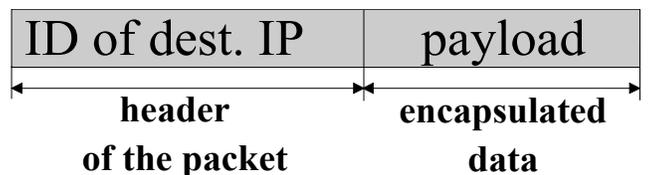
Fig. (8). Structure of the frame sent between routers and NIs.
