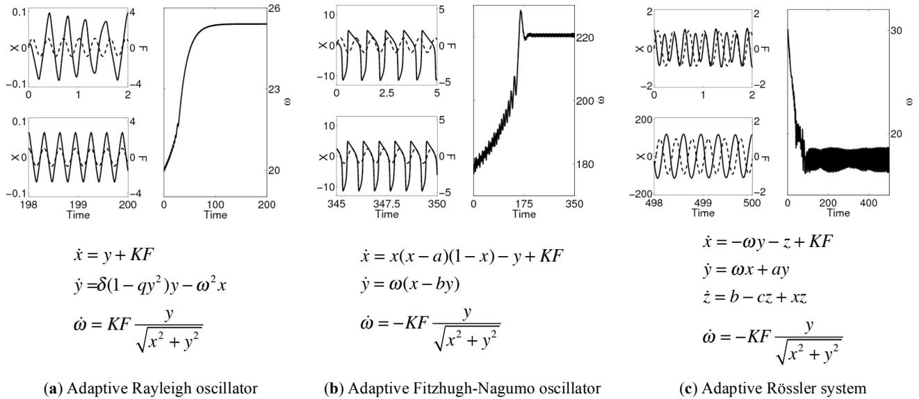
**Fig. (2).** For each oscillator,  $\omega$  corresponds to the adaptive parameter. Each figure is composed of 3 plots. The right plot shows the evolution of  $\omega$ . The left plots are the time evolution of the oscillators (the x variable) and of the input signal  $F$  (dashed line), before (upper plot) and after (lower plot) adaptation.
