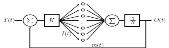
**Fig. (3).** Structure of the pool of adaptive frequency oscillators that is able to reproduce a given teaching signal  $T(t)$ . The mean field produced by the oscillators is fed back negatively to the oscillators.
