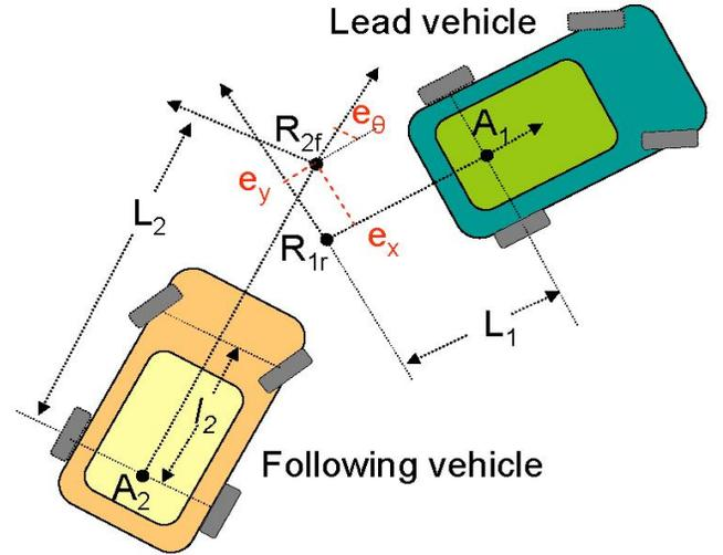
Fig. (2). System configuration for autonomous following.
