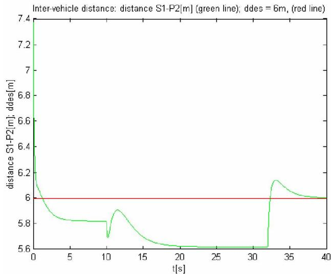
**Fig. (9).** Evolution of the inter-vehicle distance  $S_1P_2$  time (green line); Desired inter-vehicle distance during straight line motion of the leader:  $d_{des} = 6m$  (red line);  $L_1 = L_2 = 4m$ .
