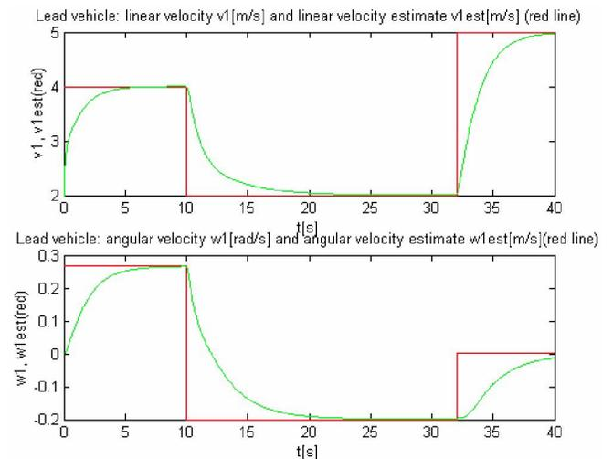
Fig. (8). Evolution in time of the lead vehicle velocities estimates ( $\hat{v}_{A1}, \hat{\omega}_1$ ) (green line); lead vehicle actual velocities  $v_{A1}$  and  $\omega_l$  (red line);  $L_1=L_2 = 4m$ ;  $d_{des} = 6m$ .
