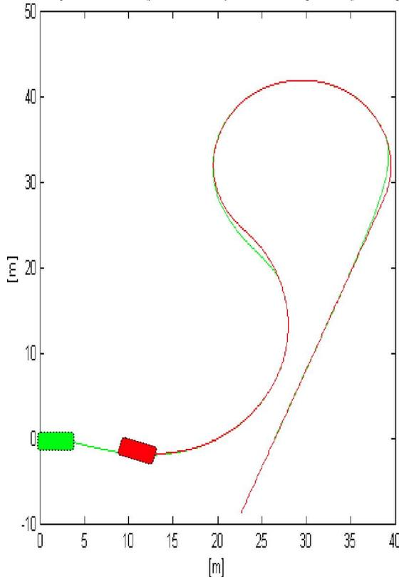
Fig. (6). A planar path down by the vehicle guide points (the mid-points of the rear vehicle axles); red line (point  $A_1$ , lead vehicle), green line (point  $A_2$ , following vehicle),  $L_1=L_2=4m$ ;  $d_{des} = 6m$ .
