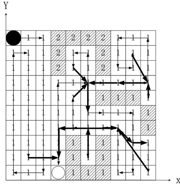
Fig. (11). the path of ISS in the environment with multiple irregular obstacles.
