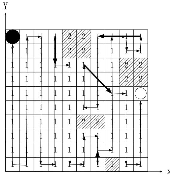
Fig. (8). The path of UAPP in the environment with multiple regular obstacles.
