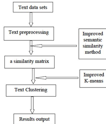
Fig. (2). Semantic clustering based on text similarity calculation.
