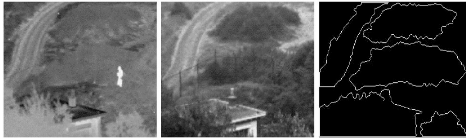
Fig. (1). Results of the image segmentation. (From left to right: infrared image, visible image and segmentation result).
