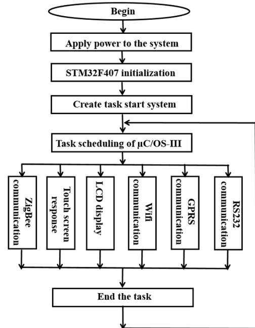
Fig. (12). Flowchart of main control system software.
