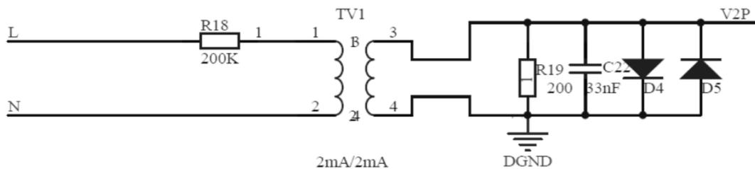
Fig. (6). Circuit diagram of voltage acquisition in the power network.
