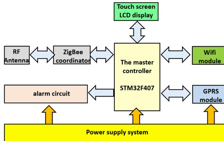
Fig. (2). Structure of the master controller.
