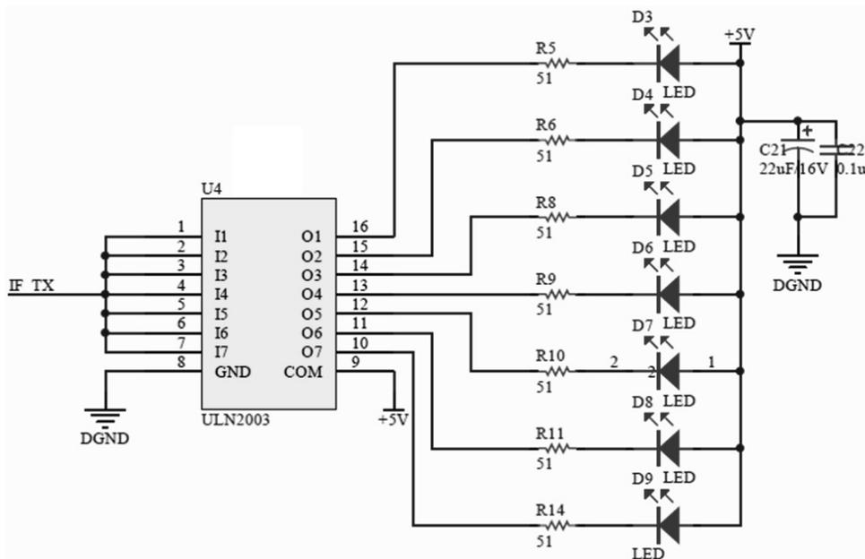
Fig. (10). Circuit diagram of infrared emitter.
