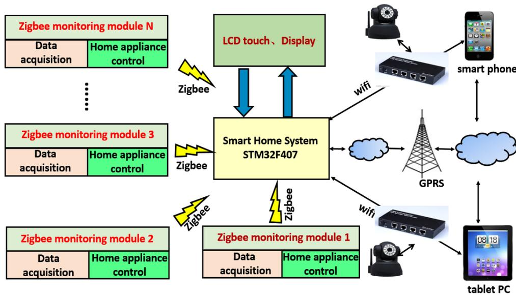
Fig. (1). Overall structure of the smart home system.
