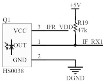
Fig. (9). Circuit diagram of infrared receiver.
