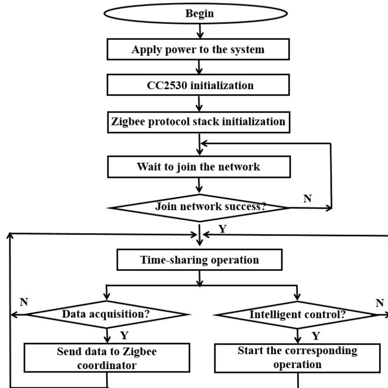
Fig. (14). Flowchart of ZigBee network node program.
