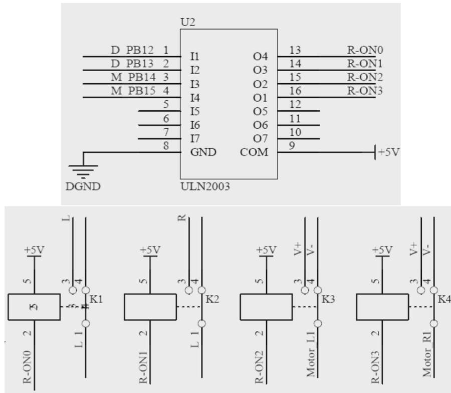
Fig. (11). Circuit diagram of electric curtains.
