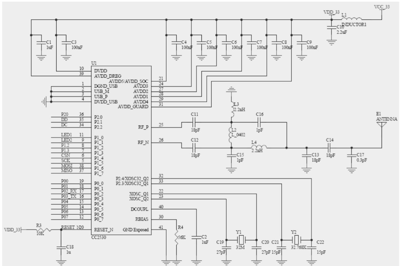
Fig. (3). CC2530 typical circuit.
