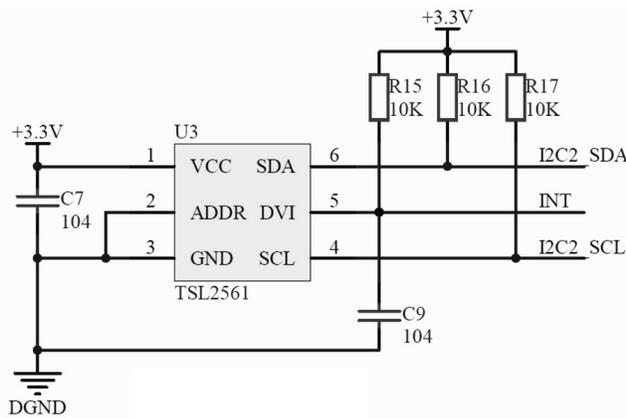
Fig. (5). Circuit diagram of light intensity sensor.
