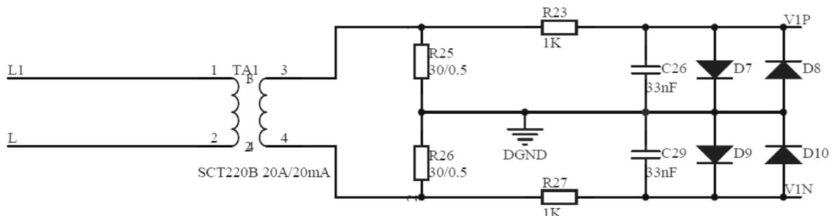
Fig. (7). Circuit diagram of the electric current acquisition in power network.
