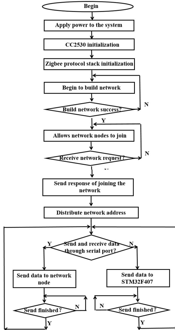
Fig. (13). Flowchart of ZigBee coordinator program.
