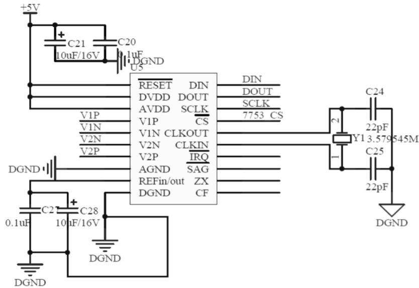
Fig. (8). Circuit diagram of ADE7753 electric parameter measurement.
