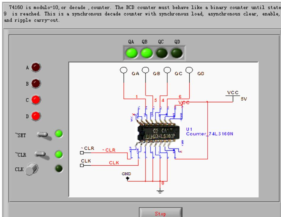
Fig. (4). Decimal counter based on 74LS160.
