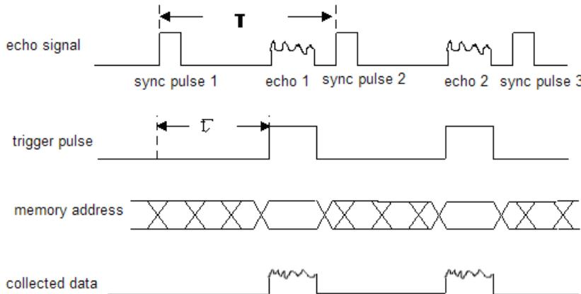
**Fig. (6).** Repeat acquisition of radar echo.
