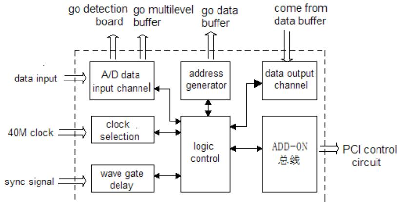
**Fig. (4).** system logic control function chart.
