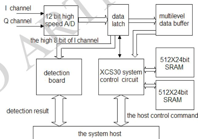
**Fig. (1).** schematic diagram of dual channel radar data acquisition system.
