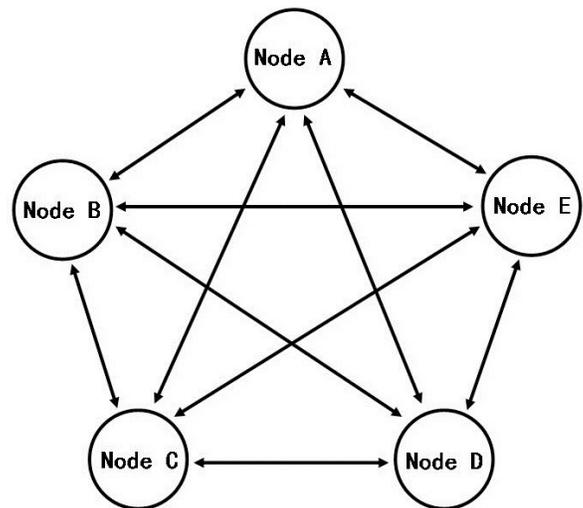
Fig. (8). Example of the Mesh Topology.
