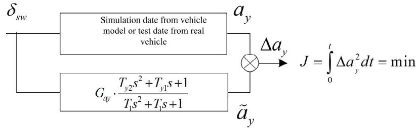
(a) The block diagram of vehicle model parameter identification
