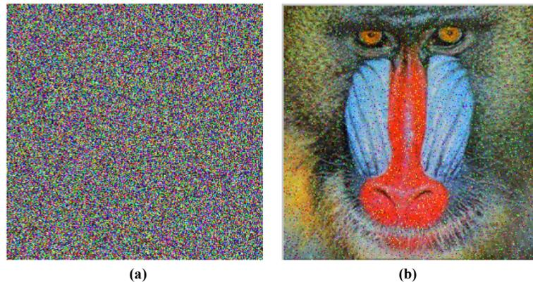
**Fig. (10).** Noise attack and reconstructed image: (a) the encrypted image with 2% Gaussian noise, (b) reconstructed image of (a).
