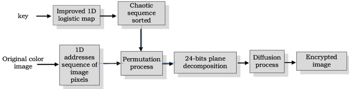
Fig. (4). The new color image encryption algorithm.
