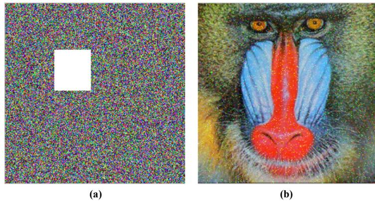
**Fig. (9).** Cutting attacks and reconstructed image: (a) the encrypted image with a 52×58 data loss, (b) reconstructed image of (a).
