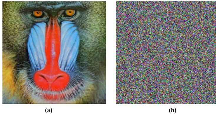
Fig. (7). Key sensitivity: (a) decrypted image with correct key={1.95164, 0.25, 8, 3}, (b) decrypted image with wrong key={1.9516400000000001, 0.25, 8, 3}.
