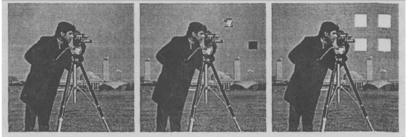
Fig. (1). A) The original image. B) The tampered image. C) The certification results of Xie method.
