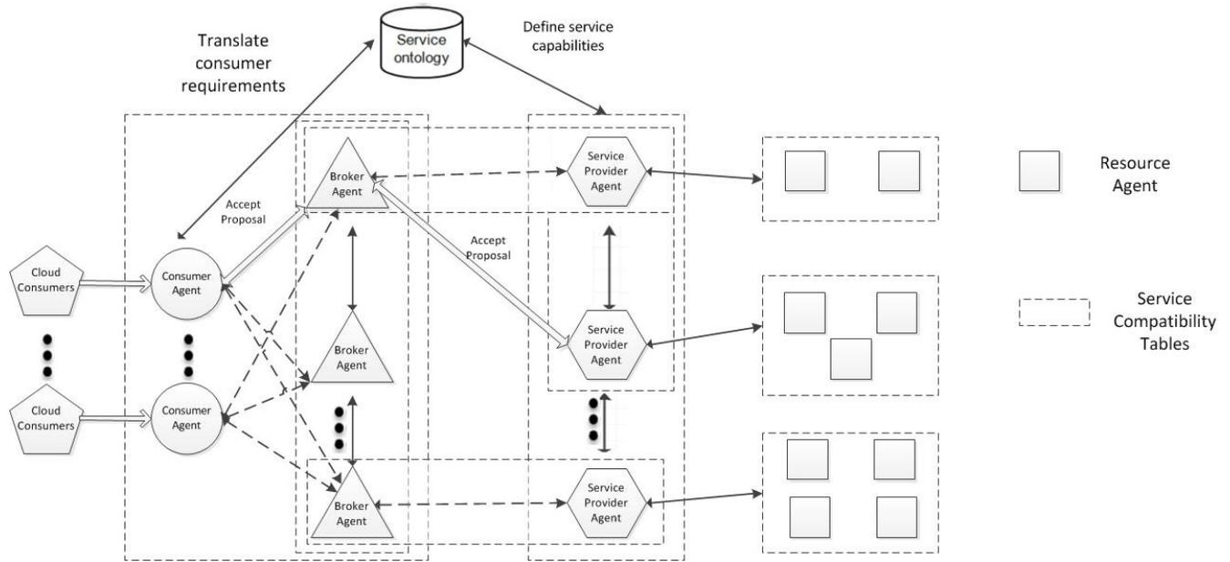
Fig. (1). Architecture of agent-based cloud computing system.
