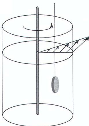
**Fig. (1).** Illustration of rotating beaker with a tablet fixed on a steel wire. The beaker is glued to the centrally placed rod at the bottom so that when the rod is rotated at fixed rpm the beaker also rotates at the same rpm (reproduced with permission from ref [46]).
