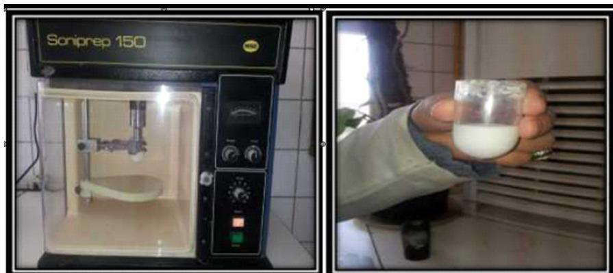
**Fig. (3).** TiO<sub>2</sub> Nanofillers were well dispersed in the monomer by a probe sonication apparatus.
