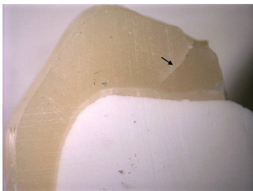
Fig. (3). Microscopic image (2.5x magnification) showing cone crack (arrow) starting at the loading area which propagates till cement layer.
