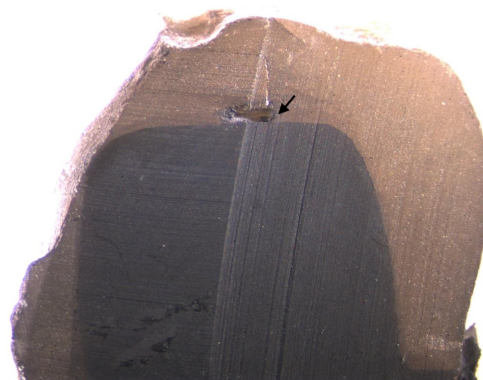
Fig. (4). Microscopic image (2.5x magnification) showing voids (arrow) within the cement layer.
