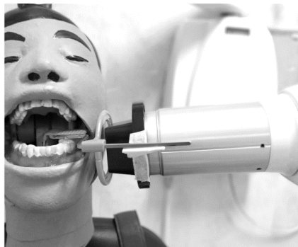
Fig. (2). Image of the phantom head (DXTR III X-Ray Trainer), composing of tissue-equivalent materials, and positioning of the tube.
