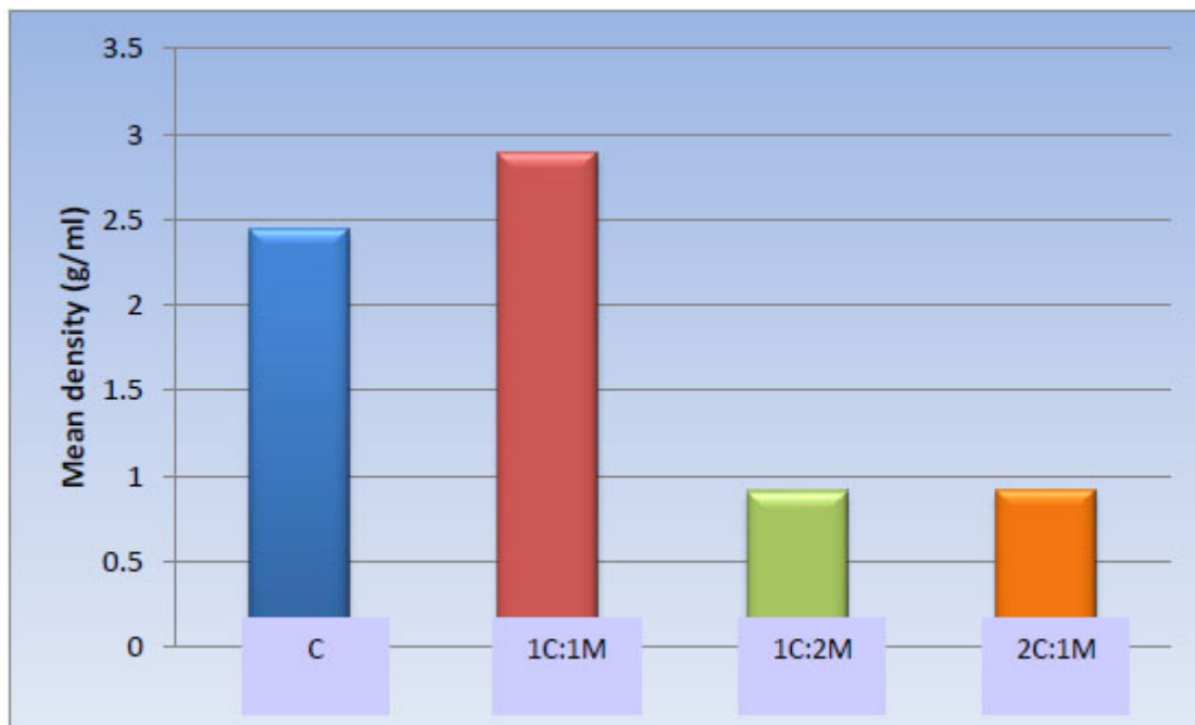
Fig. (10). Bar chart representing mean apparent [skeletal] density values [g/ml] of all chitosan-based scaffolds.
